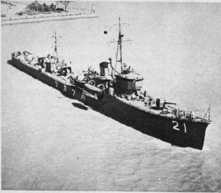
Hatsukari is one of four Chidori Class torpedo boats. These correspond to Nazi Wolf-Möwes. Chidoris and Otoris ( right ) carry three 4.7-in. guns, three 21-in. torpedo tubes and displace under 600 tons.
